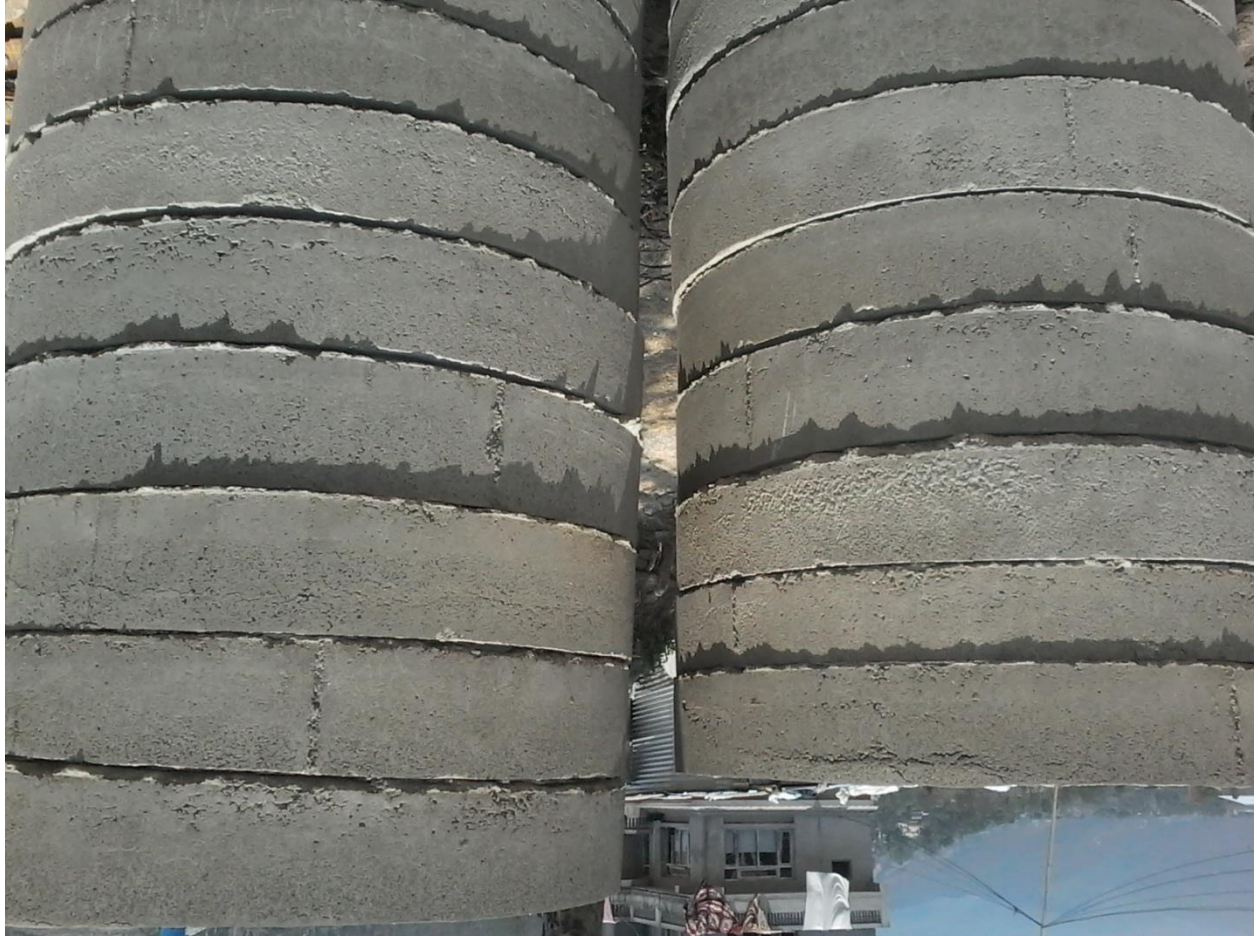
Concrete cement rings used for well construction
